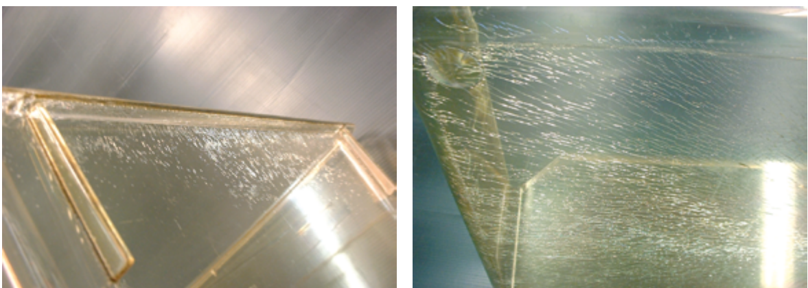
Figure 9-4 on the left a Cage body with micro cracks, on the right a detailed view of a cage body
