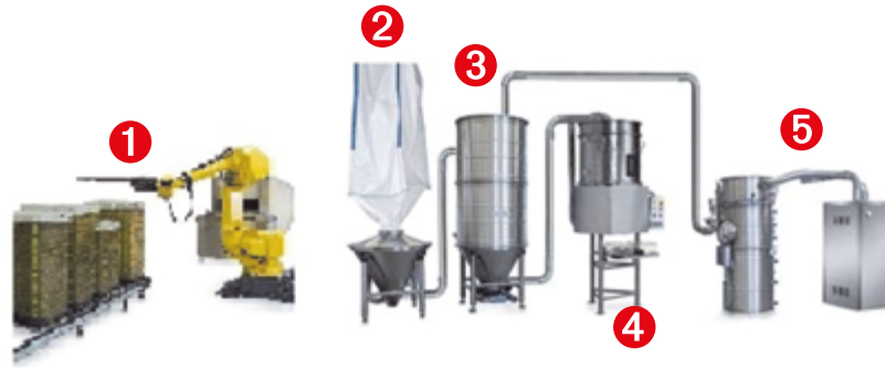
Fig. 4-17 Example for an fully automatic system: Filling of cages by robots or automatic machines ①, loading hopper e. g. for BIG-Bags ②, optional storage silo ③, dispenser with dust suction system ④ and vacuum generator and dust filter ⑤ for pneumatic conveyance
