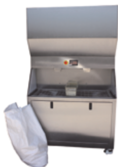
Fig. 4-15 Example for a semi-automatic system: mobile dispensing station with suitable dust suction device
