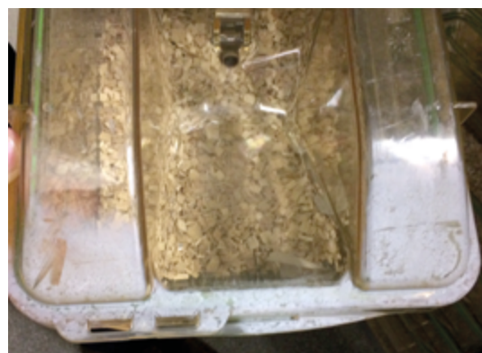
Figure 9-2 on the left a cage top and drinking bottle made of polysulfone with milky white material haze, and on the right a detailed view of a cage top
