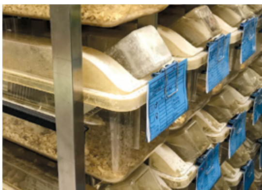
Figure 9-2 on the left a cage top and drinking bottle made of polysulfone with milky white material haze, and on the right a detailed view of a cage top
