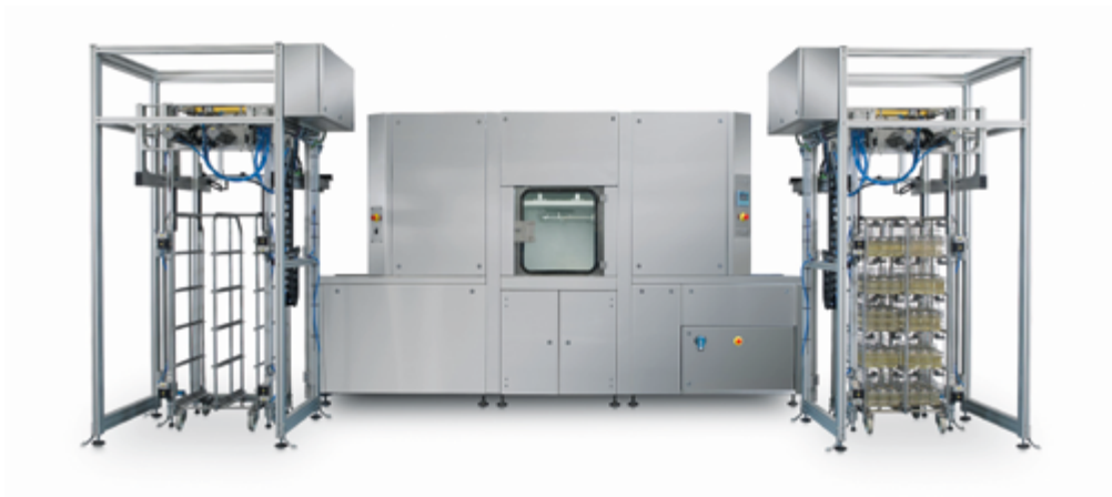
Figure 4-14 Full automated bottle washer as pass-through application, with loading from bottle crate trolley, decapper, bottle crate conveyance, washing, filling, recapper and loading into bottle crate trolley
