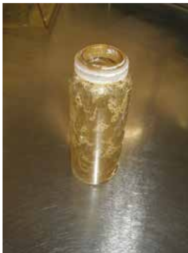
Figure 7-7 Bottle with contamination
