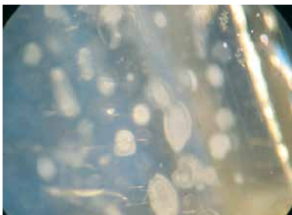
Figure 9-2 Cage parts with deposits
