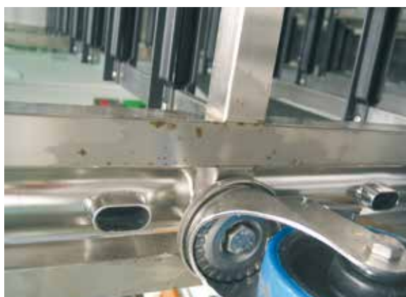
Figure 9-5 Stainless steel racks showing corrosion
