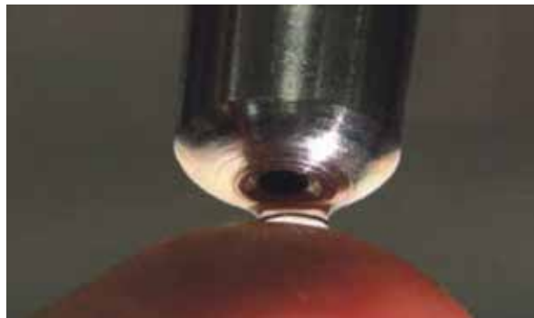
Figure 9-7 Bottle nipple with water drop (finger test to pull off the drop)
