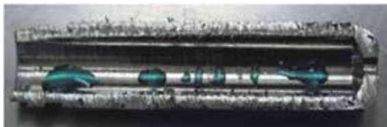
Figure 9-6 left Cut bottle nipple with inadequate water flow. Incomplete water wetting on the inner side of the capillary clearly visible
