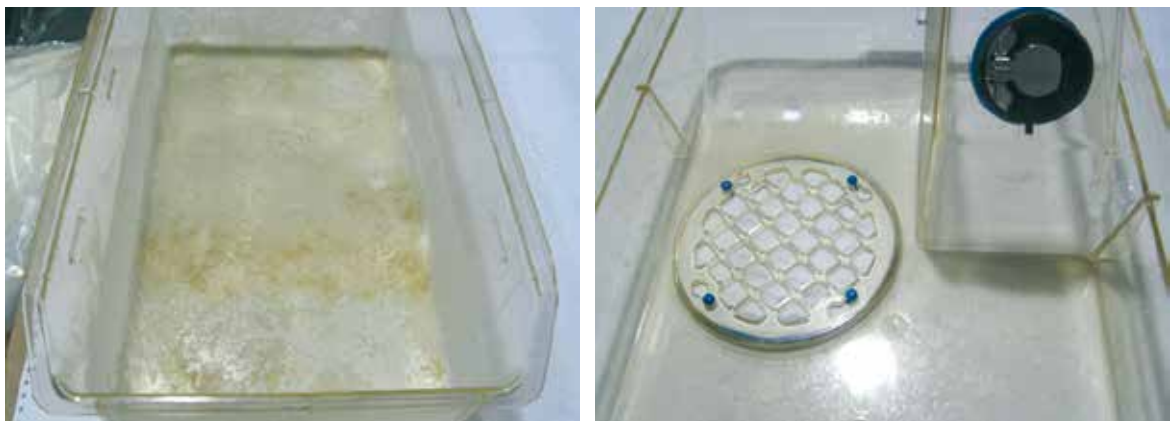
Figure 9-1 on the left a cage body, on the right a cage lid with material haze
